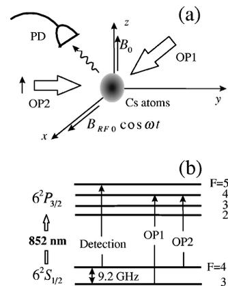
FIG. 1. (a) Schematic diagram of the experimental setup. The interaction region is in a Cs vapor cell housed in a magnetic shield not shown in the diagram. OP1 and OP2 are optical pumping beams. Detection beams (not shown) illuminate the Cs atoms from all three axes, and the fluorescence signal is detected by the photodiode (PD). (b) Tuning of the optical pumping and detection beams.
