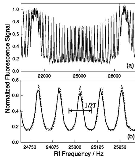
FIG. 3. (a) Ramsey resonance line shape. Data is obtained by applying two  $\pi/2$  pulses of the same duration  $\tau=0.25$  ms with an interrogation time  $T=4$  ms between them. Solid line, experimental results; dotted line, theoretical line shape, with an inhomogeneous broadening  $\Delta\omega_B/2\pi=27$  Hz and a Larmor frequency  $\omega_0/2\pi=25\,040$  Hz. (b) Magnified view of the central fringes. The FWHM of the central fringe is 36 Hz, and is much narrower than  $1/2T$ .
